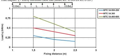
Specified load ratings are independent of splice plate location.
