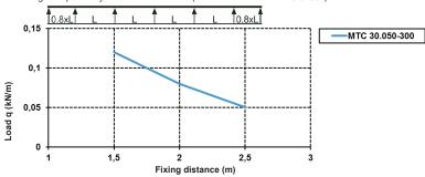
Specified load ratings are independent of splice plate location.
